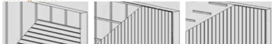
Horizontal installation : vertical battens
